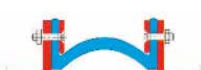
Profile II Installed by means of angle flanges and backing flanges. For positive pressure.
