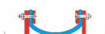
Profile III Installed by means of angle flanges and backing flanges. For negative pressure.
